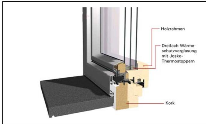
The ChristophorusHouse is a passive house and therefore, it has no heating in the conventional sense. So in the planning and during all construction phases, special attention had to be paid to the airtight condition of the building. Windows are of course the critical spots in this respect. Completely newly developed solid wood passive house windows were used for the first time in such a large size passive house and they ensure a maximum of energy preservation in the ChristophorusHouse.
